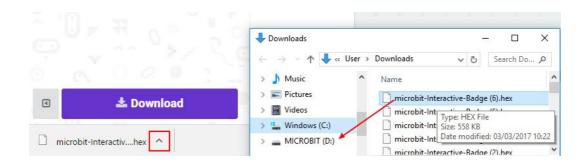
A light on the back of your micro:bit will flash while the file is being copied. Once this has stopped your program will run. You can click the reset button on the back of your micro:bit to restart the program.
